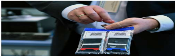
A radiation dosimeter used for individual monitoring in IAEA laboratories. (Photo: D. Calma/IAEA)
